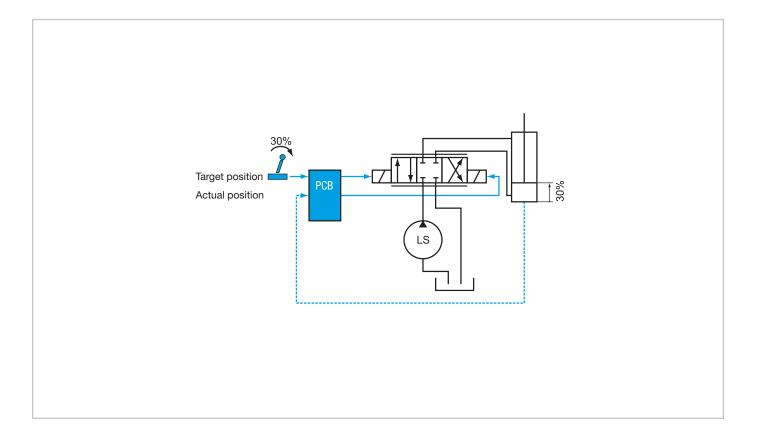
Position controller PCB [connection example]
